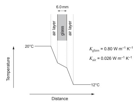
I. Use the rate of heat loss through the window to show that the temperature difference across the glass is approximately 0.3 °C. [2]
